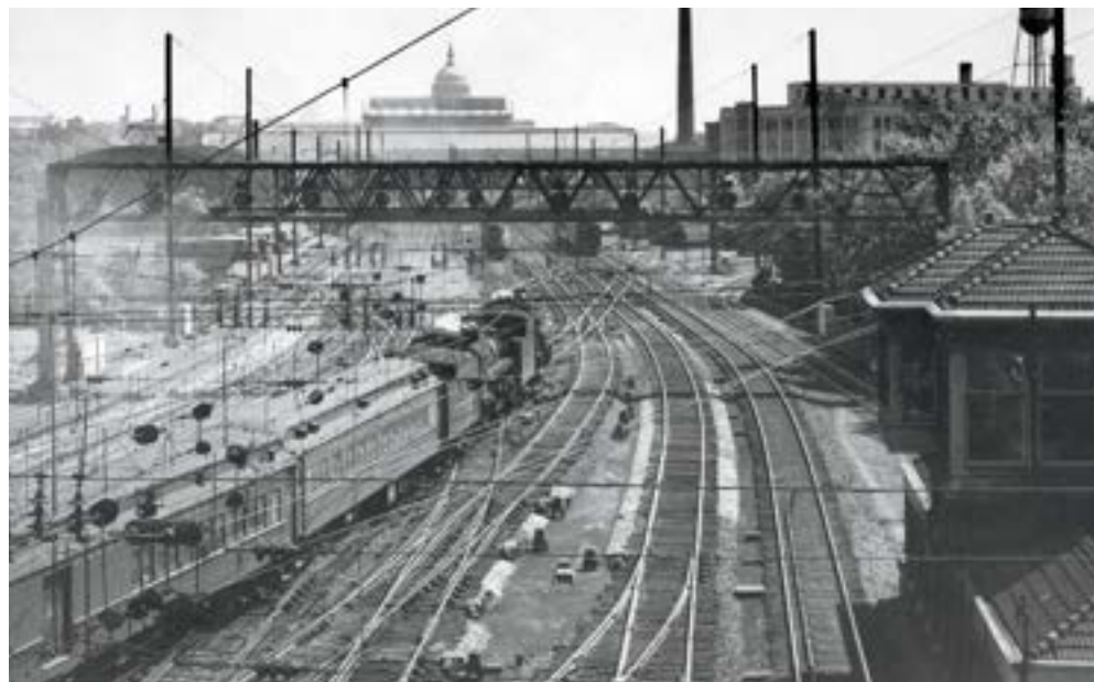
Washington: Doubleheaded 4-6-2s on a Royal Blue Line train approach Washington Union Station, beyond which rises the U.S. Capitol dome, in May 1937. The two tracks closest to the tower at right are B&O's Metropolitan Division from Harpers Ferry, W.Va.
