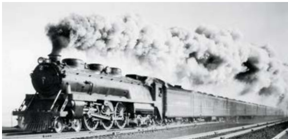
Watertube-fireboxed 4-6-4 Lord Baltimore — one of B&O motive power boss George Emerson's experiments — has the original lightweight Royal Blue in hand at Elizabethport, N.J., in 1937, shortly before the engine and cars were reassigned to the Alton. R. P. Morris
