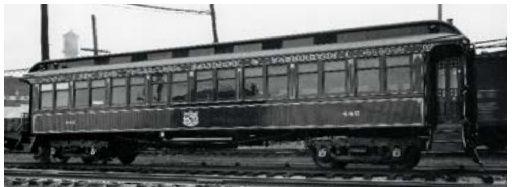
In a thrilling 1905 publicity photo (top), Royal Blue Line trains pass at speed on famous Thomas Viaduct outside Baltimore. B&O vestibule coach 445 (above) of 1896 is resplendent in dark blue with gold lettering and striping and Maryland's coat of arms.
