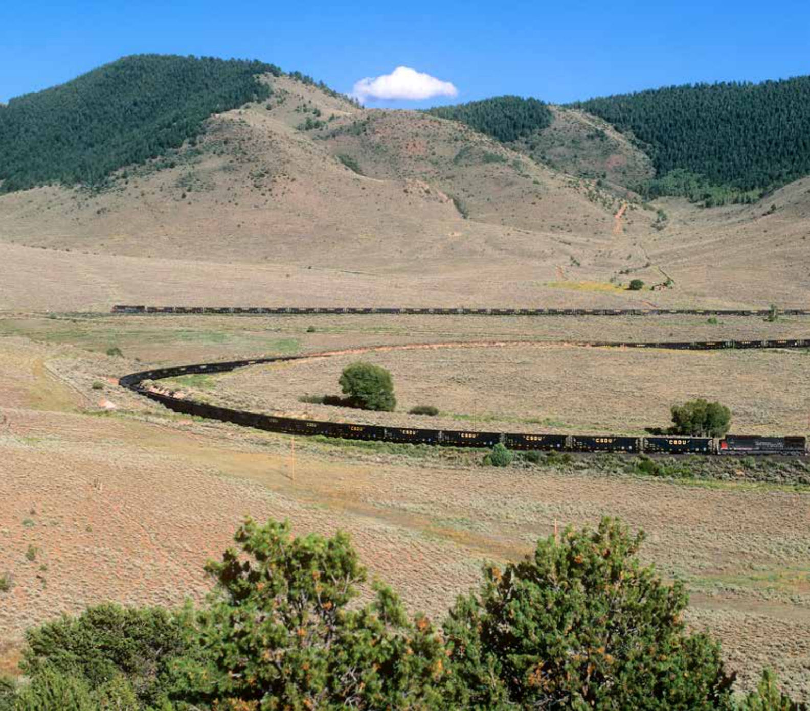
A Southern Pacific coal empty climbs through the loops at Crater, Colo., on July 30, 1996. A single AC4400CW, No. 298, leads the train, with two mid-train distributed power units out of sight and two more, Nos. 361 and 226, bringing up the rear.
