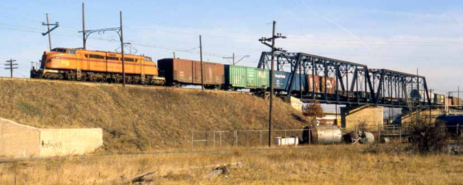
In 1949, South Shore purchased three of 20 massive 2-D+D-2 “Little Joes” built by GE for the Soviet Union but never delivered. No. 803 leads a westbound freight over the Penn-Wabash bridge in Gary. Lou Gerard
