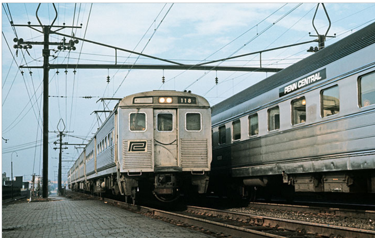
New Jersey Arrow MU cars and a Budd all-roomette sleeping car rebuilt as a coach illustrate the range of equipment deployed by PC in commuter service on the Northeast Corridor. Jim Heuer
