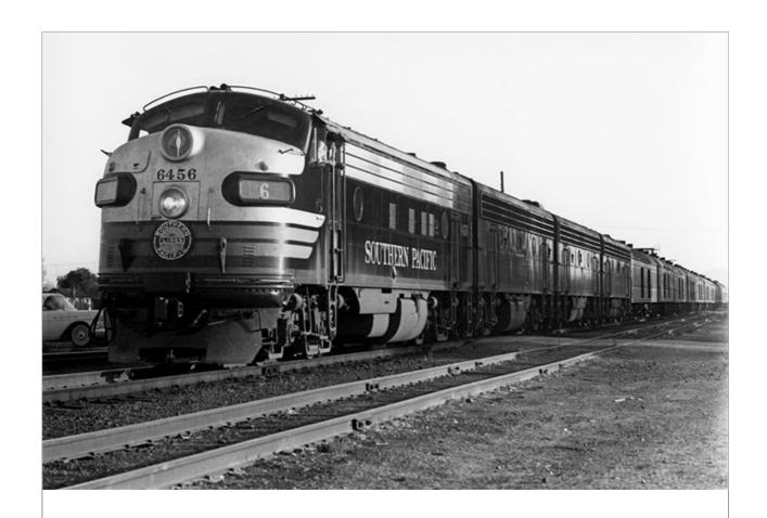
Led by an SP FP7A in the railroad's revered "black widow" scheme—black, silver, and orange—the eastbound Argonaut at Wilcox, Ariz., on April 20, 1958 shows about a dozen head-end cars in front of the passenger-carrying section. The Argonaut spent a large part of its life obscured by the Sunset. M. D. MC Carter, Thad Carter collection
