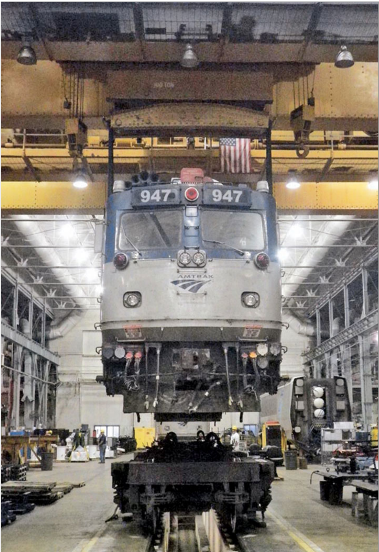
AEM7 947 is being lifted off its wheels and will be placed on a work stanchion near-by. This unit is slated for a rebuild. Mark Florio
