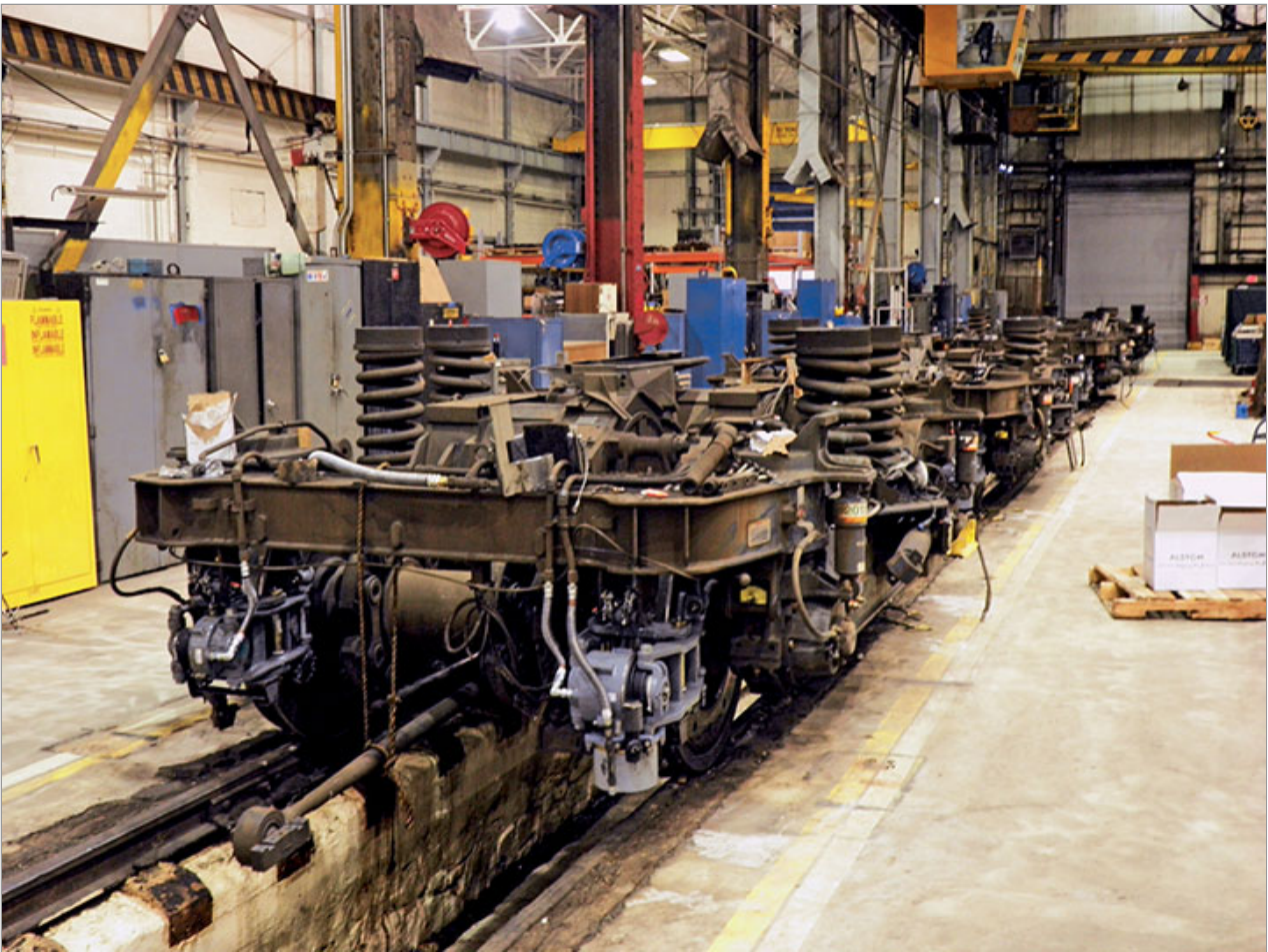
The lower wheel and frame assembly of AEM7 947 sits on the shop floor awaiting its overhaul and rebuild. Mark Florio
