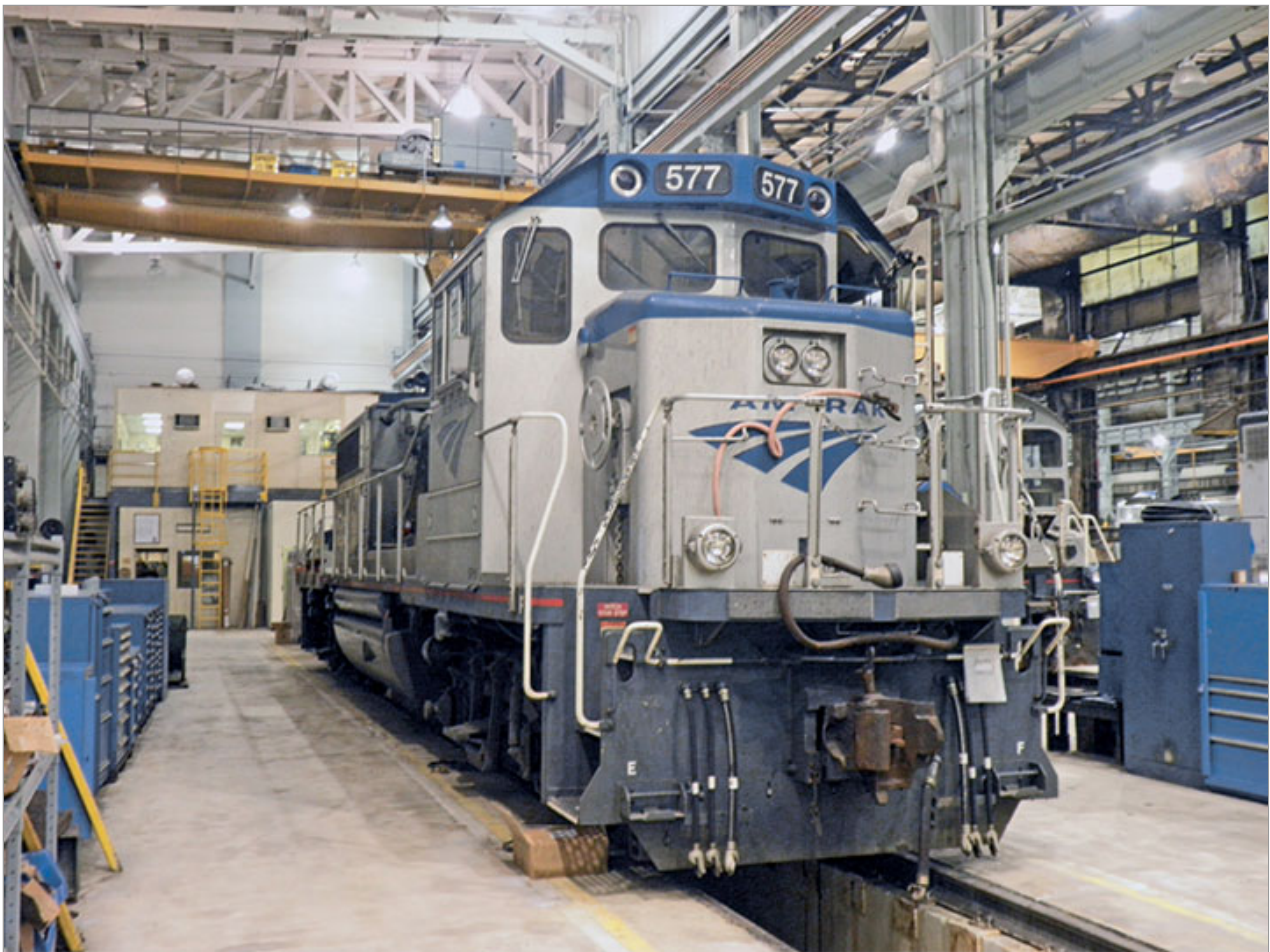
Amtrak maintenance-of-way locomotive GP15D No. 577 sits on the pit track awaiting its regular servicing and inspection. Mark Florio
