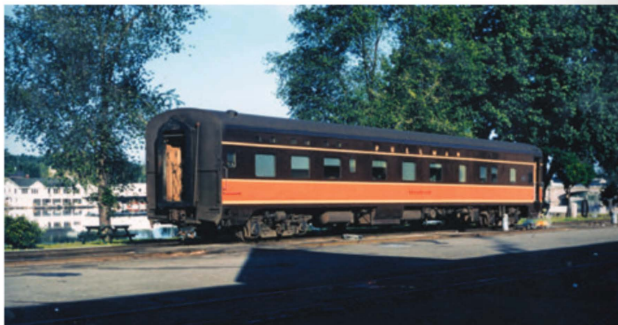
RIGHT So far, this is the only known photo of the Hawkeye 's set-out sleeper—on this day the Sugarland , a 6-6-4 sleeper built by Pullman-Standard for Panama Limited service in 1942—at Waterloo, Iowa, dropped by train 11. It was photographed on June 2, 1966. Set-out sleeper service between Chicago and Waterloo ended early in the 1960s. JOHN HUMISTON, RICHARD HUMISTON COLLECTION
