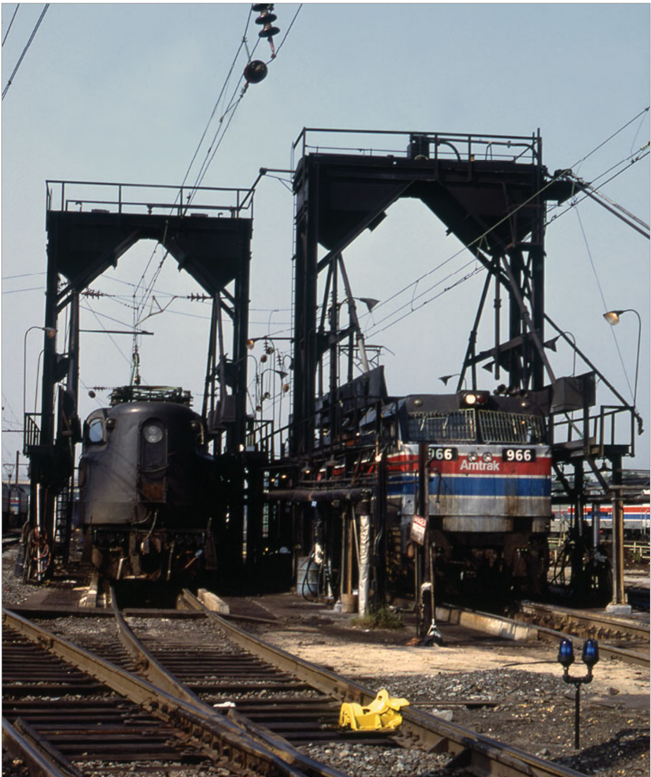
Amtrak used former Penn Central GG-1s and newer E60 electric locomotives on its Northeast Corridor trains. Here one of each locomotive type sits at the servicing towers in the Ivy City shops.
