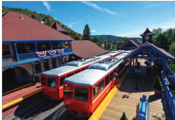
ABOVE: This photo taken at the Manitou Springs station shows the difference between the more traditional outside rail and the cog rail in the middle, which helps propel the train uphill. JUSTIN FRANZ PHOTO
