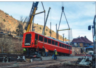
ABOVE: While the railway was completely rebuilt, the four SLM diesel-hydraulic rail car sets were shipped out for new Strub cog rail use and had their Cummins small cam 855 engines upgraded to large cam ones for more horsepower. Originally, all railway equipment was conveyed on streetcar tracks that connected to rail lines, which were torn up in 1930s. Now, everything is trucked in, as evidenced by a car being lowered into the Manitou Springs yard with cranes before the resumption of service in May 2021. COURTESY OF BROADMOOR HOTEL
