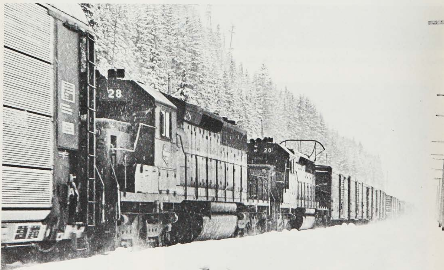
PANTOGRAPH-LIKE deflector atop lead slave SD40-2 knocks off icicles in advance of trilevel cars.
