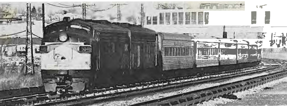
FL9 STILL BEARING NEW HAVEN LOGO ON AMTRAK'S SALT CITY EXPRESS Leased diesel-electric-electrics handle the Harmon-Grand Central leg
