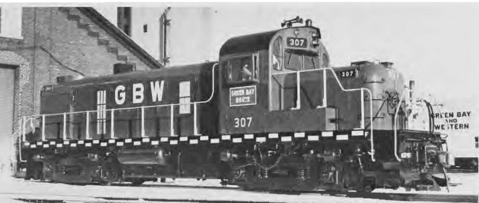
GB&W 307 FRESH OUT OF NORWOOD SHOP WITH 2000 H.P. ALC WHITE V-12 251-C Only a few ALC loyalists are giving old 244 models renewed life.
