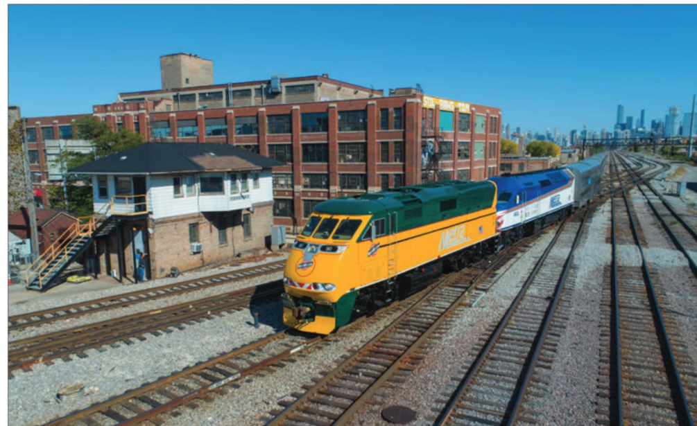
BELOW: Metra C&NW heritage unit F59PHI 90 leads an M7901-07 passenger extra into UP's California Avenue Coach Yard, situated just west of Tower A-2. The purpose of some of the plant's double-slip switches is shown in this westbound move from UP Track 2 into the Fence Track for the yard.
