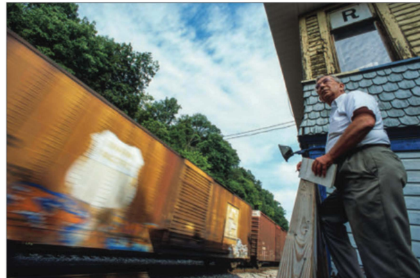
RIGHT: Paul Swain inspects a westbound at Miller Tower on July 23, 2000. Any defects he may find will be noted on his pad and reported to the dispatcher and train crew. Operators were an extra set of eyes, adding to the safe passage of a train.
