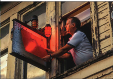
ABOVE: At West Cumbo, Carl Kief demonstrates the use of the B&O's unique order board on August 1, 1997. If a train is to stop for orders, a red light is turned on and a red metal plate is hung on the board. For orders on the fly, a yellow light and yellow plate are used.
