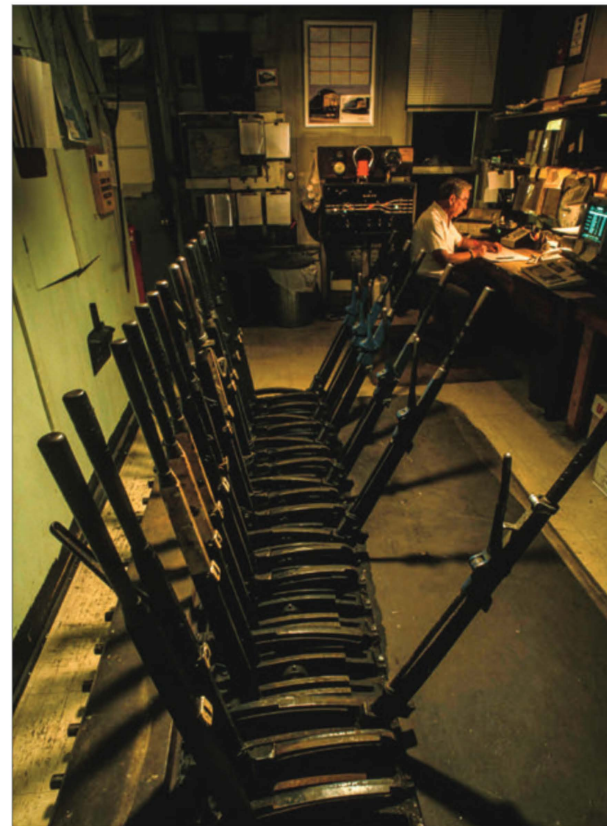
LEFT TOP: A relatively modern touch in the last string was the pistol-grip levers at West Cumbo. Operator George Speis is framed by a window there on August 25, 2000.
