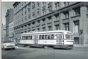
ABOVE: On a day nearly as dark as the future of Montreal's PCC fleet, MTC 3511 passes a sister on the Outremont Line. The shells were built at St. Louis Car Co., with final assembly taking place in Montreal at Canadian Car & Foundry. BRUCE BATTLES-LTL
