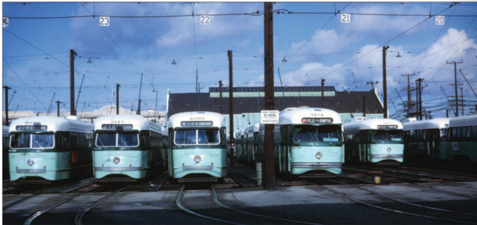
ABOVE: The narrow gauge 42-inch trackage of the former Los Angeles Railway is clearly evident in this head-on view at the Georgia Street yard of Los Angeles Metropolitan Transit Authority. Remarkably, the yard consists of elevated track above a "pit" adjacent to a city street. Note the differences in car widths between PCC 3090 (100 inches) to the left of the pole and PCC 3151 (108 inches) to the right. It's March 1963, and the end of PCC service in Los Angeles is only days away. BRUCE BATTLES-LTL
