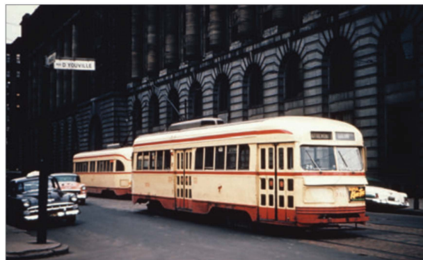
ABOVE: On a day nearly as dark as the future of Montreal's PCC fleet, MTC 3511 passes a sister on the Outremont Line. The shells were built at St. Louis Car Co., with final assembly taking place in Montreal at Canadian Car & Foundry. BRUCE BATTLES-LTL
