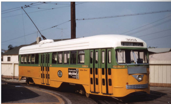
ABOVE: The narrow gauge 42-inch trackage of the former Los Angeles Railway is clearly evident in this head-on view at the Georgia Street yard of Los Angeles Metropolitan Transit Authority. Remarkably, the yard consists of elevated track above a "pit" adjacent to a city street. Note the differences in car widths between PCC 3090 (100 inches) to the left of the pole and PCC 3151 (108 inches) to the right. It's March 1963, and the end of PCC service in Los Angeles is only days away. BRUCE BATTLES-LTL
