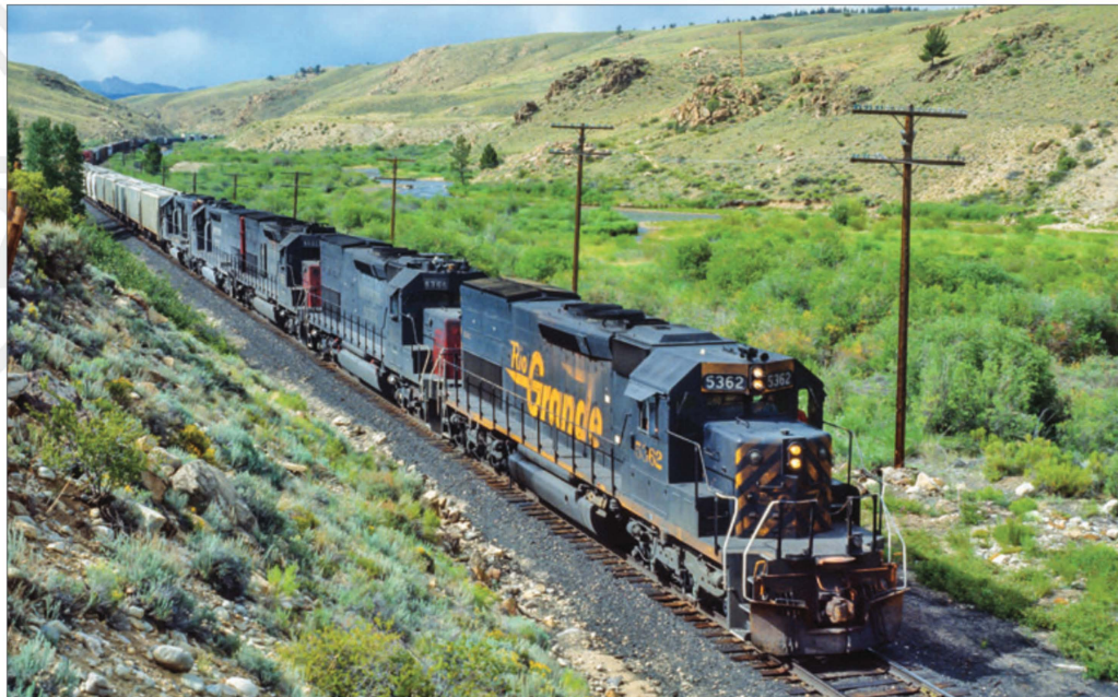
ABOVE: Pushers on the rear of an eastbound coal load are at Winter Park, Colo., in August 1994, site of the Moffat Tunnel west portal. The 5407, an SD40T-2, is cleaner than its fellow helper engine.
