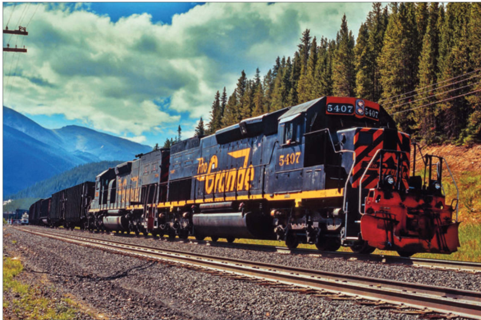
ABOVE: Pushers on the rear of an eastbound coal load are at Winter Park, Colo., in August 1994, site of the Moffat Tunnel west portal. The 5407, an SD40T-2, is cleaner than its fellow helper engine.
