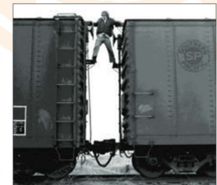
BELOW: Conductor George Napoleon releases high hand brakes at Hickman as stored PFE mechanicals are readied for the trip to Stockton on January 27, 1977. TED BENSON PHOTO
