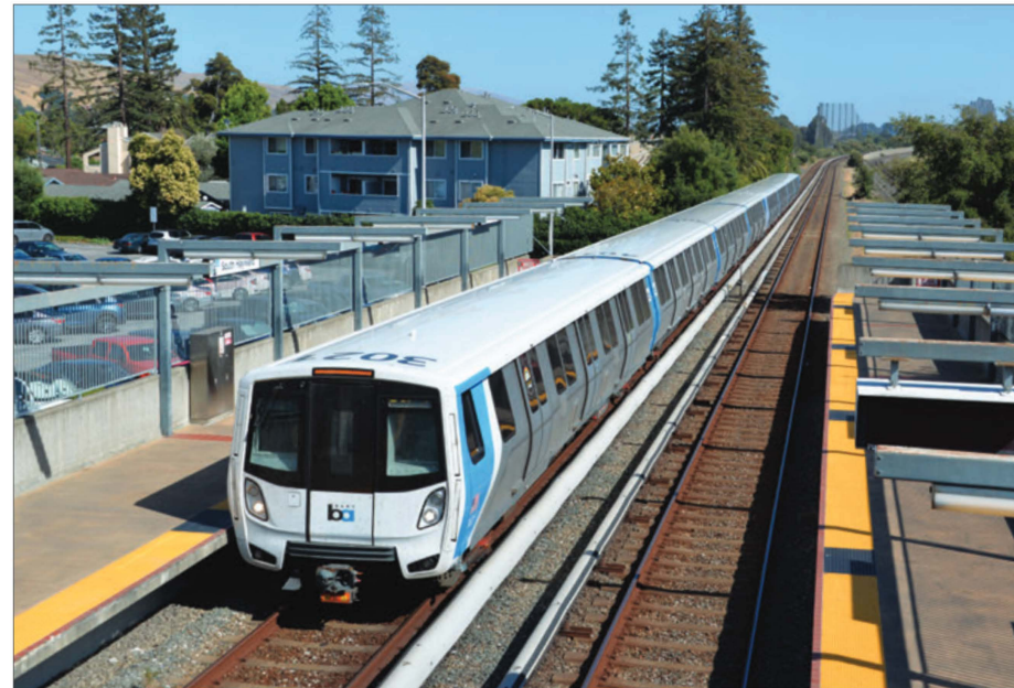
BELOW: At South Hayward, 10 FOTF cars glide into the station in July 2019. D-car 3021 leads the way, followed by eight E-cars and another D-car in the "trail position," as BART designates that role. The 775 Bombardier FOTF cars will not work in multiple with other members of the BART fleet. As deliveries of these cars increase fleet size, older members of the BART system will be retired. GORDON LLOYD JR./ANTHONY J. SCHILL - LTL
