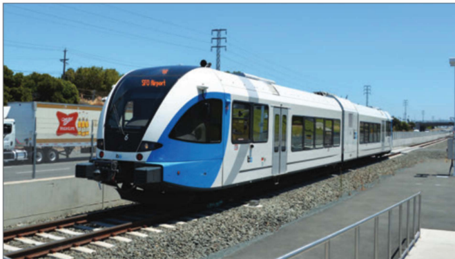
LEFT: BART's extension to Antioch, known as eBART, is an anomaly. The standard-gauge line uses Stadler GTW diesel multiple-unit equipment. A cross-platform transfer at Pittsburg/Bay Point affords patrons an additional 10 miles of highway avoidance. GORDON LLOYD JR.-LTL
