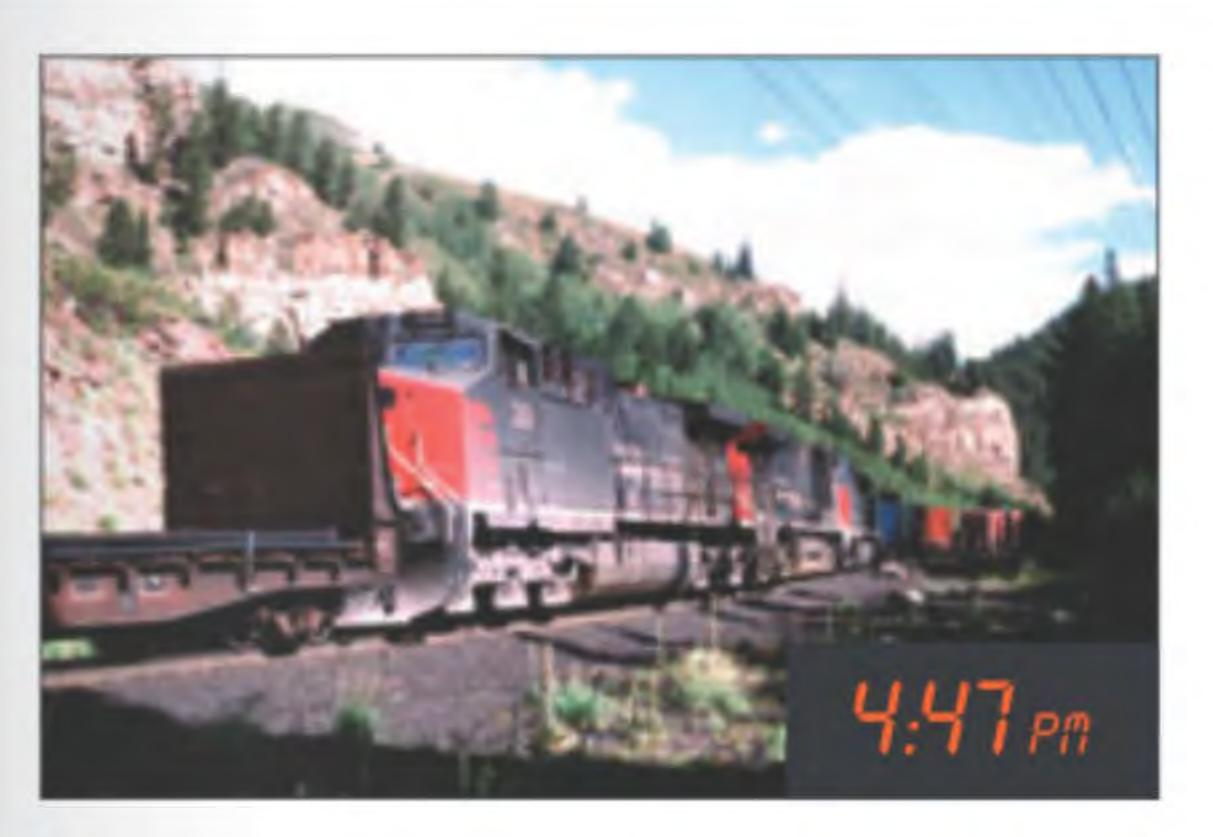
ABOVE: Third movement — Stillwater, halfway between Belden and Pando, mile 291.7. Eastbound Train RVKCM-5, with four tunnel motors in charge, heads up the pass through a seldom-seen remote valley of the Eagle River. With three ACs cut in mid-train, the train is sufficiently powered to maintain a posted 25 mph speed up the 3 percent grade at full throttle. At Pando, 1.5 miles ahead, the engineers will throttle back on the 1–1.7 percent grade to keep the speed in check.
