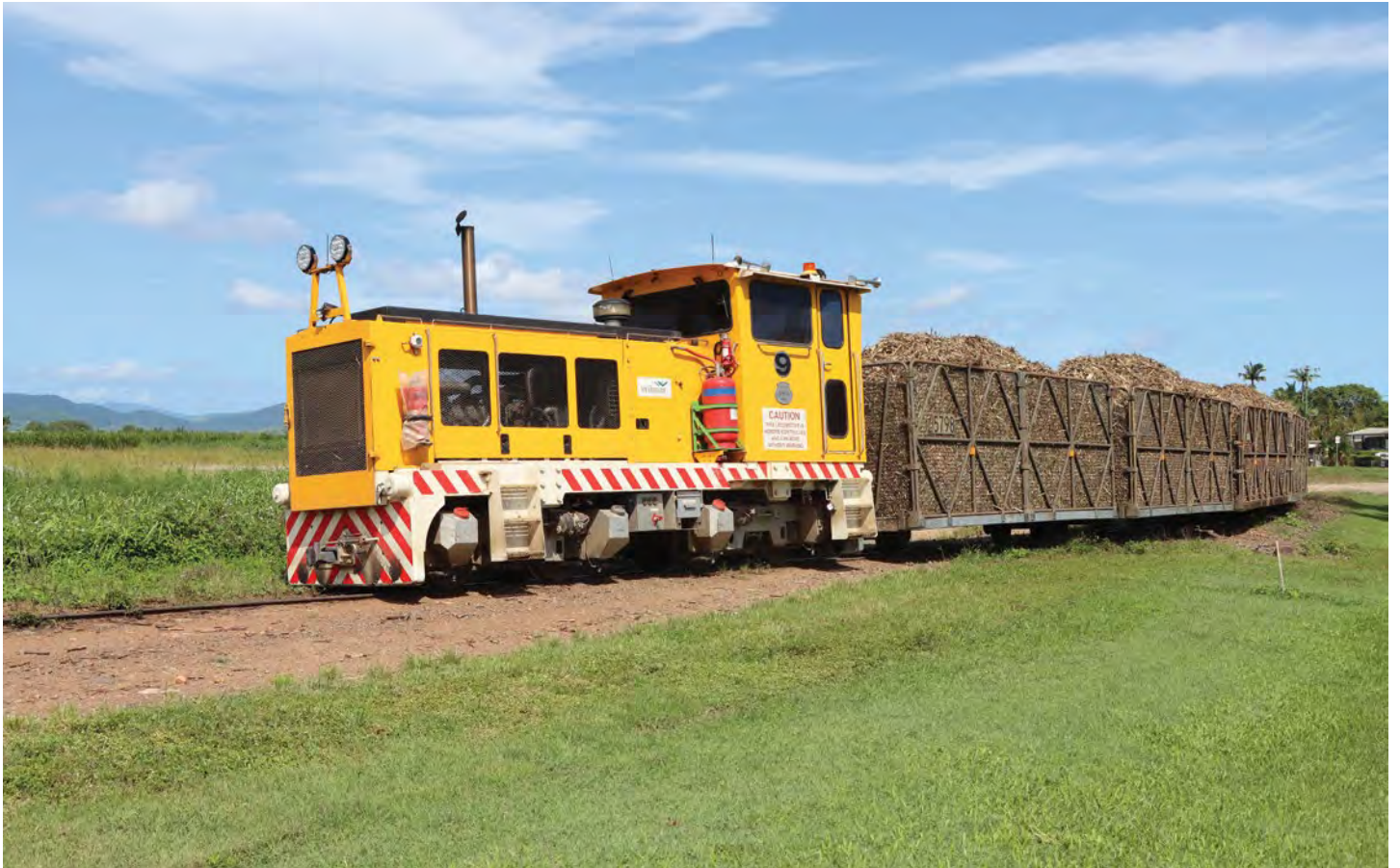
Above: EM Baldwin B-B DH number 9 picks up some full 10 tonne Bins from Mackay Corner, clearing the way for EM Baldwin number 10 to deliver some empty 10 tonne bins, on Sunday 8 January 2023. The notice on the cabside reads "CAUTION This locomotive is remote controlled and can move without warning". Luke Horniblow
