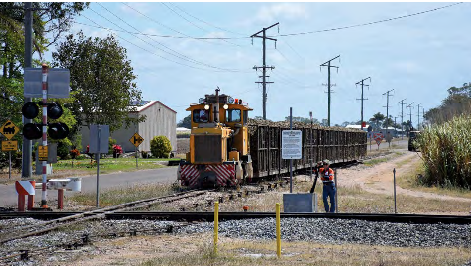
Kalamia Mill's Comeng 0-6-0DH Delta has just collected a short train of loaded cane bins and is proceeding across Queensland Rail's North Coast Line at the McDesme Cane Train Crossing beside Giddy Road at McDesme, 5km south of Ayr, on Saturday 30 September 2023. The sign behind the lever gives step-by-step instructions on how to safely operate the crossing. Stephen Whitaker
