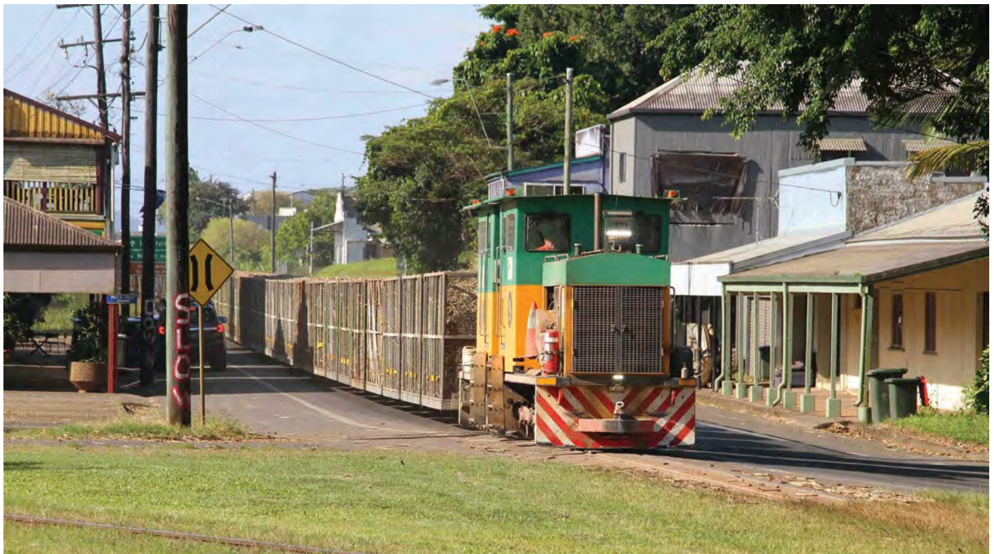
Mid-afternoon on Wednesday 22 September 2021 finds coupled Comeng 0-6-0DH pair 9 and 8 rolling a loaded cane rake from the north past the delightfully ramshackle shopfronts of Hynes Street, South Johnstone. The train is only a coin toss from the front bar of the Criterion Hotel, on the left, and the mill is a few hundred metres ahead. Malcolm Holdsworth
