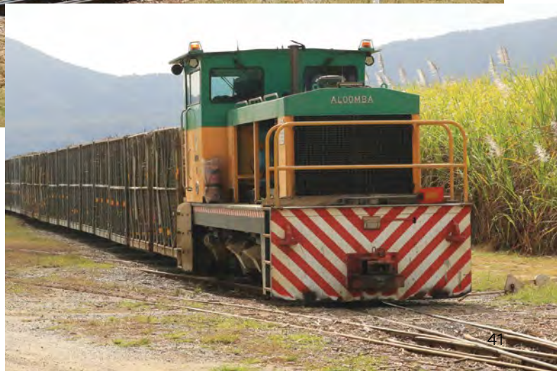
Above: The difference in height between the Walkers B-B DH locomotives and the 'low-cab' Clyde 0-6-0DH units is demonstrated in this scene near the mill on Sunday 25 September 2022 as Redlynch , hauling a loaded train, overtakes Mulgrave . James Chuang
