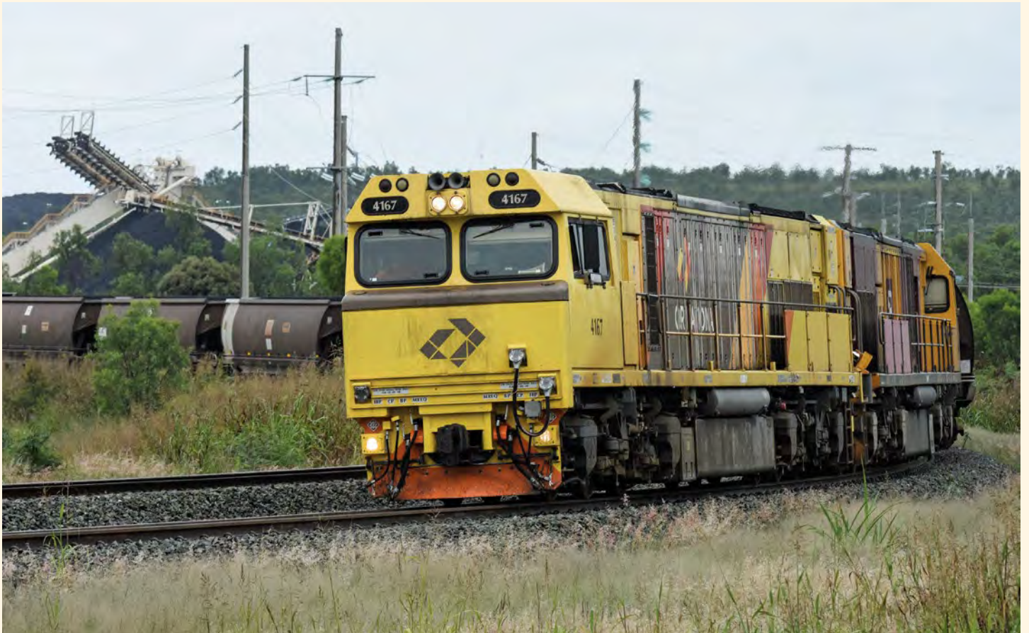
Above: A combination of Aurizon and QR liveries is commonplace on the Moura System, as seen here on Sunday 15 January. With the aid of mid-train units 4165 and 4036, Aurizon loco 4167 and QR liveried 4007 ease their loaded train around the balloon loop at the Moura (Dawson) mine before departure for the Port Of Gladstone. Other balloon loops are utilised at Boundary Hill, Callide and Baralaba mines.
