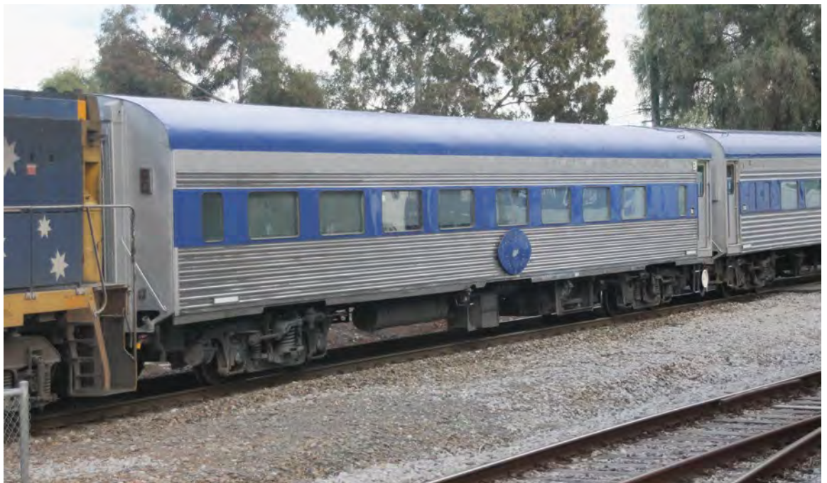
Journey Beyond Rail Expeditions on the Overland use the South Australian Railway Workshops built Pullman-Standard style Cor-Ten cars. These cars were built with stainless steel fluting on the body sides. BJ 6 is the lead car on the eastbound Overland passing the Adelaide suburb of Mitcham on Friday 1 September 2017. John Beckhaus
