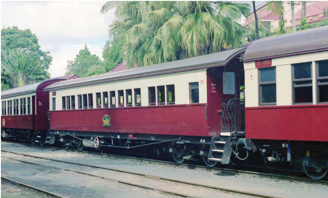
BLH 752 was built during 1913 as a longitudinal seat Davidson car. It was rebuilt during 1936 as a side aisle car. BLH 752 was at Kuranda station on Sunday 30 July 2006. John Beckhaus
